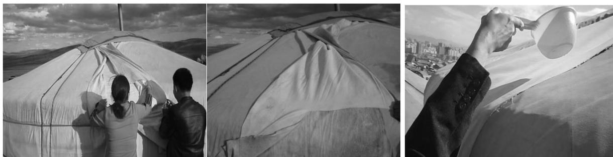
Fig. 7 Water repellence test in yurt cover material
