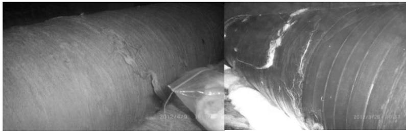
Picture 1 Damage of a shaft coating
