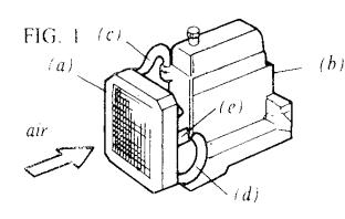
Most car engines are cooled by water. The water flows around the *engine* and then passes through the *radiator*. It then passes through the water pump and around the engine again.
